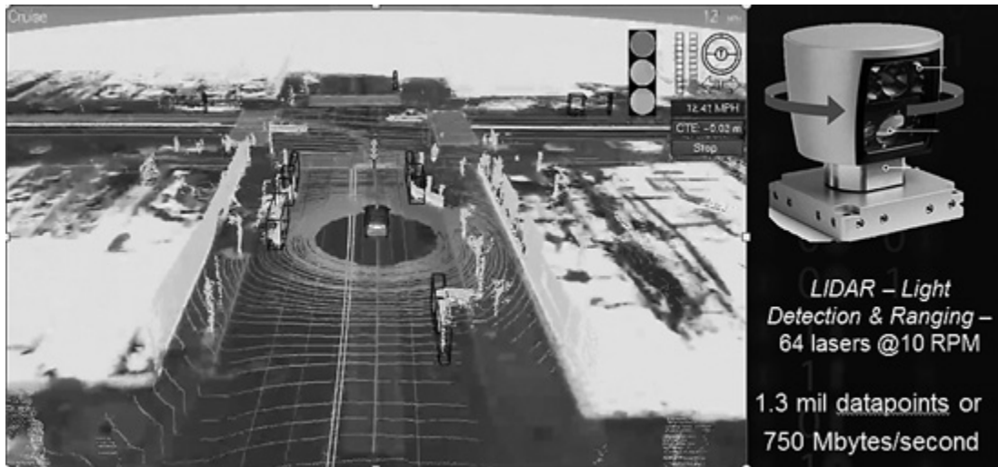
360-degree LIDAR imaging in Google's driverless car
